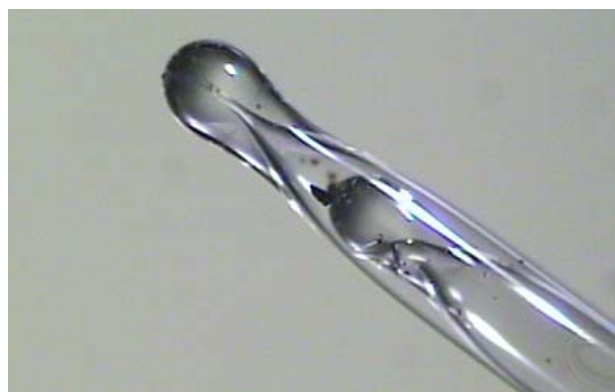
Figure 6.2. A picture of a single crystal of \text{Gd}_5\text{Ga}_{1.0}\text{Ge}_{3.0} prepared for high temperature X-ray diffraction experiments.
